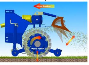
By means of our patented roller pendulum system, you can easily control the operating depth. As a unique bonus, we have provided the scarifying machine with a hydraulic adjustable cover. This is ideal when you are required to scarify near the edges and corners of a pitch.
