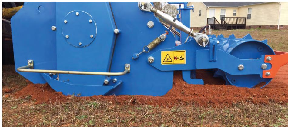
The Stoneburier is a premium rotary tiller, in which the strainer behind the rotary tiller ensures that the stones get separated from the finely crumbled ground. It is possible to equip the rotary tiller with two different types of tilling blades. Because of this operation the stones will be put under the layer of fine, vital soil.
