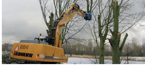
With the grapple, you can grab the trunk of the tree in the precise place where you want to cut it off. The grapple is equipped with a hydraulically powered Hardox blade, which is designed to cut trunks up to 45 cm, depending on the version of Lumberjack you have. The machine has four orbital engines that control a tooth clutch and, in conjunction with the movement of the excavator, once you have cut off the trunk, you have the freedom to inspect the tree through 360°.
