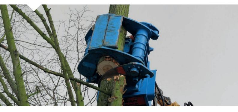
Grubbing trees in an urban area or the thinning of forests can demand some precision work. Ideally, you want to be able to cut off the entire tree and transport it to a safe area for sorting or putting through a chipper shredder. The Lumberjack will enable you to clear the trees in the safest and most efficient way. Together with the Lumberjack you are in immediate possession of a felling head and sorting machine.
