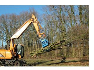
The felling head can function as a sorting machine. When you choose not to work with the cutting function it will not negatively affect your work. Nevertheless, when you do need the cutting function, you can immediately use it again.
